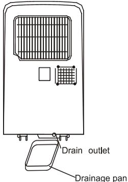
To empty the water, switch the unit off by pressing the ON/OFF button, wait for three minutes, and then disconnect from the mains supply. Place a drainage pan underneath the drain outlet plug (an the bottom of the unit, at the back in the centre). Withdraw the bung, and allow the water to drain into the drainage pan. Replace the bung, and reconnect the unit to the mains supply.
