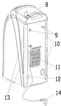
Stand the appliance on a firm, flat, level surface, at least 500 mm from the nearest wall.
