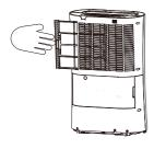
1. CLEAN THE GRILLE AND CASE Use water and a mild detergent to clean the washable mesh filters. Do not use bleach or abrasives. Do not splash water directly onto the main unit. Doing so may cause an electrical shock and can lead to the insulation to deteriorate, or cause the unit to rust. The air intake and outlet grilles get soiled easily, so use a vacuum attachment or soft brush to clean. Wipe the dehumidifier body with a soft damp cloth or kitchen towel.
