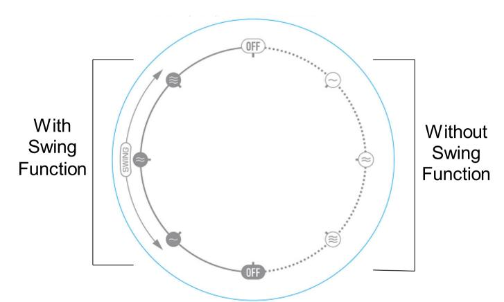
Twist the dial to select the desired fan speed, following the table below, twisting to select operation with or without the swing function.
