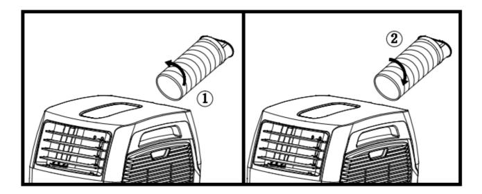
The hose can be removed by screwing the hose anti-clockwise (2)
