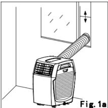
**Note:** The window kit is only designed to be installed with sliding or sash windows or doors. The window kit is not designed or to be used with any other style of windows. However the fish tail adaptor can be used with most windows / doors.
