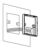
Pass the signal wire through the opening in the rear of the backing plate, ensuring it is positioned so it will not be trapped or damaged during installation. Allow enough cable to pass through for ease of installation and future maintenance.
