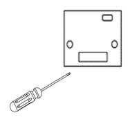
Remove the wired controller from the backing plate using a flat headed screwdriver in the gap between the backing plate and the controller. Once the two parts are separated, the remainder can be unclipped.
