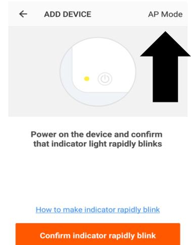
4. Ensure the WIFI light on the air conditioner is slowly flashing (once per three seconds), then press on the orange button at the bottom of the screen to confirm
