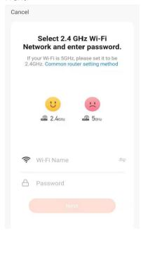
4. Ensure the WIFI light on the air conditioner is flashing twice per second then press on the orange button at the bottom of the screen to confirm
