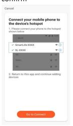
6. Go to network settings in your phone and connect to the "SmartLife xxx" connection. There is no password to enter. Then return back to the app to complete setup.
