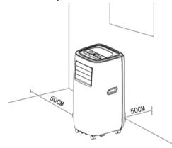
3. Make sure the unit is upright and there are no obstructions to the air inlets and outlet grills.
