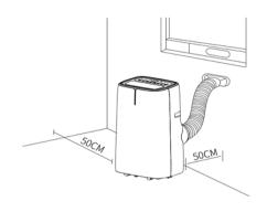
3. Make sure the unit is upright and there are no obstructions to the air inlets and outlet grills.
