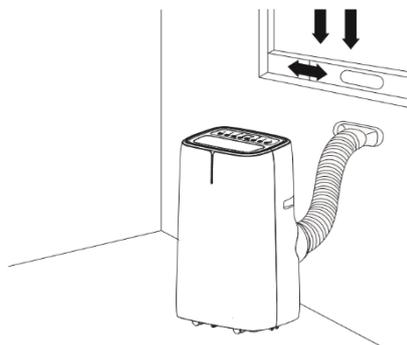
2. Fix the fishtail adaptor into the opening on the slide bar
