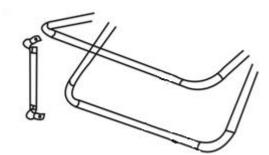
2. Slide the Axle rod through the Mounting Bracket, before attaching a wheel to either end of the Axle using an Axle Cap Nut at each end to secure them.
