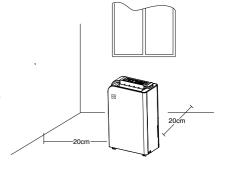
moisture as soon as it is turned on. Excess moisture is dispersed throughout your home. For this reason, the dehumidifier should be positioned in a central and clear location so that it can draw this moist air towards it from all over the home. A warm hallway or landing is an ideal position for your dehumidifier. If possible, leave interior doors ajar to allow air circulation between rooms.
