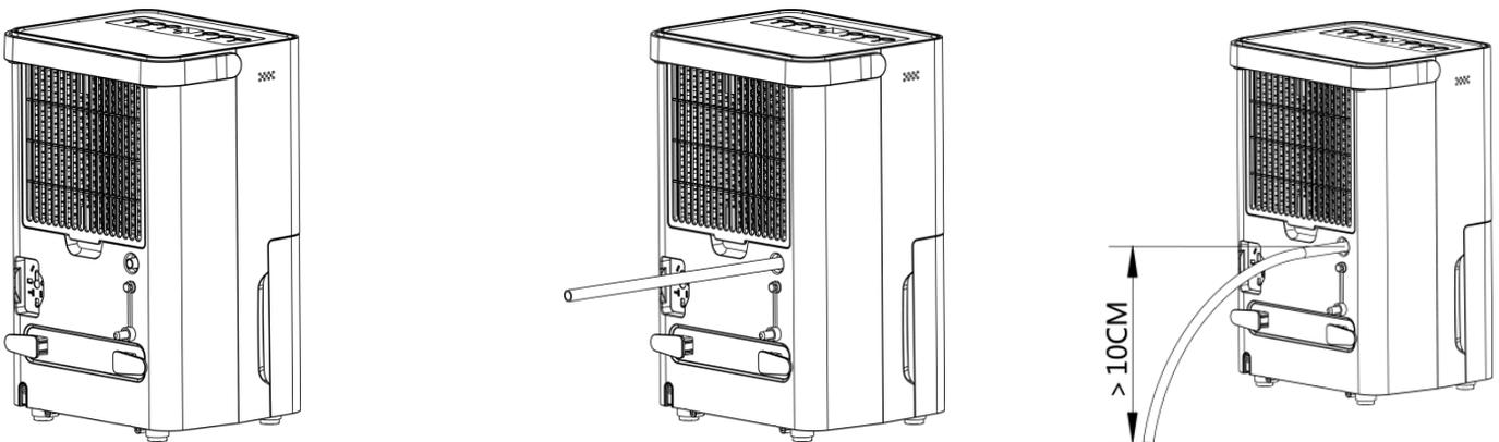
Make sure the connection between pipe and the drain outlet is tight and does not leak. Then direct the pipe to a suitable drainage point. This unit uses gravity to dispose of water hence the drain should be lower than the water outlet on the unit. Put the tank back. Be sure to run the water pipe downward and let the water to flow out smoothly. Do not kink or bend the pipe.
