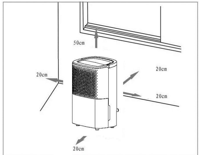
Your electriQ dehumidifier will begin to protect your space from the harmful effects of excessive moisture as soon as it is turned on. Excess moisture is dispersed throughout your home. For this reason, the dehumidifier should be positioned in a central and clear location so that it can draw this moist air towards it from all over the home. A warm hallway or landing is an excellent position for your dehumidifier. If possible, leave interior doors ajar to allow air circulation.
