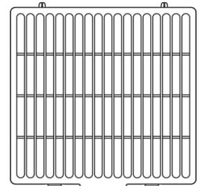
Remove the filter frame. If the optional carbon filters are fitted, remove them from the frame and Hoover gently approximately every 2-3 weeks.
