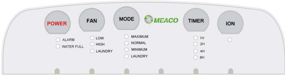
**Power** - Lights up when there is power to the dehumidifier, the unit beeps three times when it is turned on.
